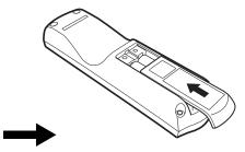
If all buttons on the remote control do not light when the [LIGHT] button is pressed, or buttons are inoperative when you attempt to operate the projector, replace new batteries.
